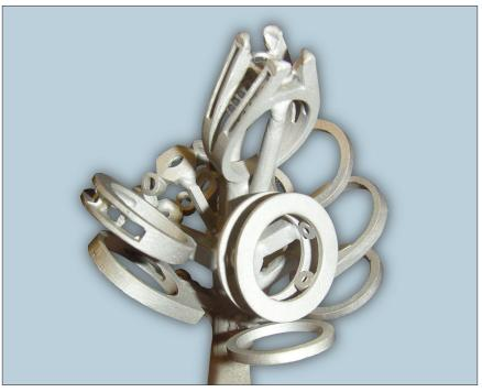
There was a noticeable decrease in micro gas porosity in the white gold castings, without a tremendous increase in surface finish in the as-cast state. This is likely due to the investment's ability to decrease sulfur dioxide formation at the metal mold interface during casting.
