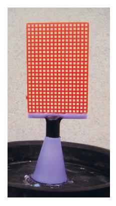
In the experiments conducted at AU Enterprises, wax grids, plates, and trees, as well as rapid prototype models, were cast using the Ultra-Vest MAXX investment.
