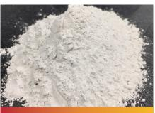
Zircon is almost exclusively used in the primary slurry and as a primary stucco. Because of its high density, zircon provides excellent flow characteristics in a primary slurry. The round grains do not cause defects such as rough casting surfaces.
