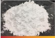
Ranco-Sil fused silica can be used throughout the ceramic shell. When used in the primary slurry, it may be necessary to blend with zircon depending on the alloy. Shells constructed with fused silica hold their dimensions better and are not prone to hot deformation or bulging. Shell removal from the casting, or knockout, is also easier with fused silica refractories.
