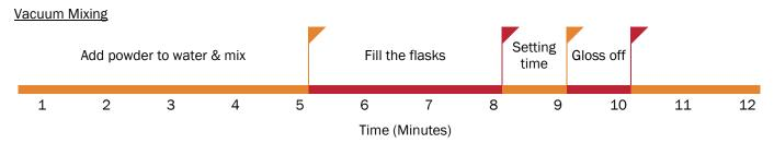
Work time: Elapsed time between adding powder to the water and thickening of investment.
