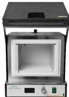
Vulcan single-stage burnout furnace
