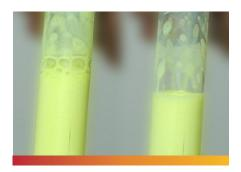
DCH-10 antifoam is a water-based silicone emulsion used in colloidal silica based slurries to reduce air entrapment.
