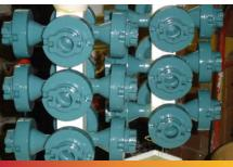
R&R Wash-N-Etch pattern cleaner also acts as an etching material for the wax pattern while it cleans off the release agent. This process allows for better slurry adhesion during application of primary coats. Better adhesion of the primary coats reduces opportunities for casting defects related to shell buckling or lifting.
