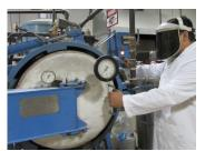
It is recommended that the autoclave be operated to at least 100 psi. The temperature inside the autoclave will be about 340°F (171°C). Comparing the pressure and temperature readings will let you know that both are functioning properly.
