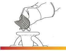
On contact with molten metal, the surface fibers of Pyrotek High Temperature Glasweve™ filters form a sticky layer of fayalite. This allows the fabric to remove even micron-sized inclusions from the beginning of the pour to the end.
