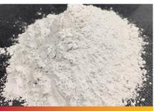
Zircon is almost exclusively used in the primary slurry and as a primary stucco. Because of its high density, zircon provides excellent flow characteristics in a primary slurry. The round grains do not cause defects such as rough casting surfaces.
