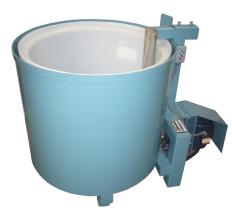
Manufactured by Pacific Kiln & Insulations Co., Inc. (PKI), the economy slurry mixer is simple, safe, durable and affordable. It is a contamination-free, rotating tub slurry mixer at a budget price, where simplicity means easy maintenance and less downtime.
