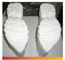
A high expansion, extra strength shoe mold plaster that produces detailed replications and consistent sizing for aluminum shoe molds.
